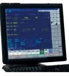
All functions appear as color icons on the LCD monitor screen for simple operation, even for inexperienced users.
