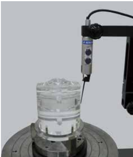
Sample roundness measurement of outside diameter
