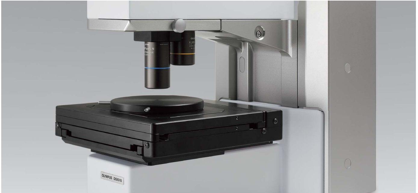
Motorized stage with 100 mm × 100 mm stroke
