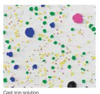
(Ductile cast iron showing nodular graphite)
