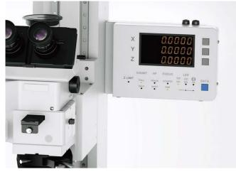
Digital readout attached to the frame
