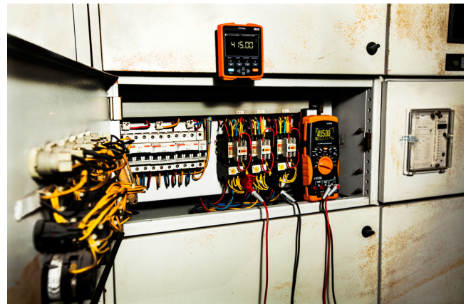
Figure 3. Monitoring handheld meter readings via the U1115A remote logging display
