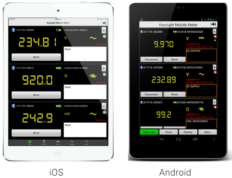
Figure 9. Up to three handheld meters measurements with the Keysight Mobile Meter Application
